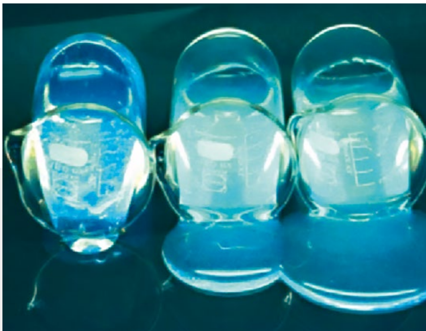
Ladder study of varying dosages of ADDITOL® VXW 6388 RHEO
