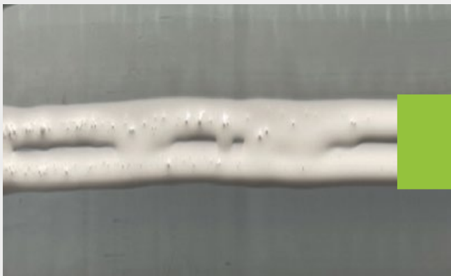
Sagging of paint on vertical substrate
