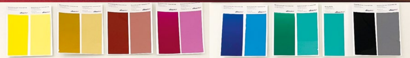
Full shade and white reduction with colorants based on ADDITOL® XL 6557 DISP
