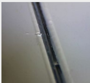
Air drying paint without drier on drying recorder
