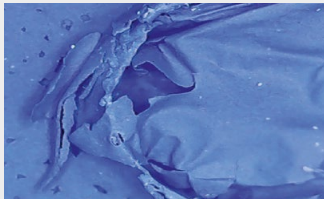
Microscopic picture of ruptured foam bubble
