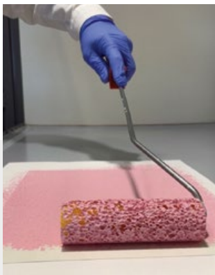
Defoamer evaluation via roller application
