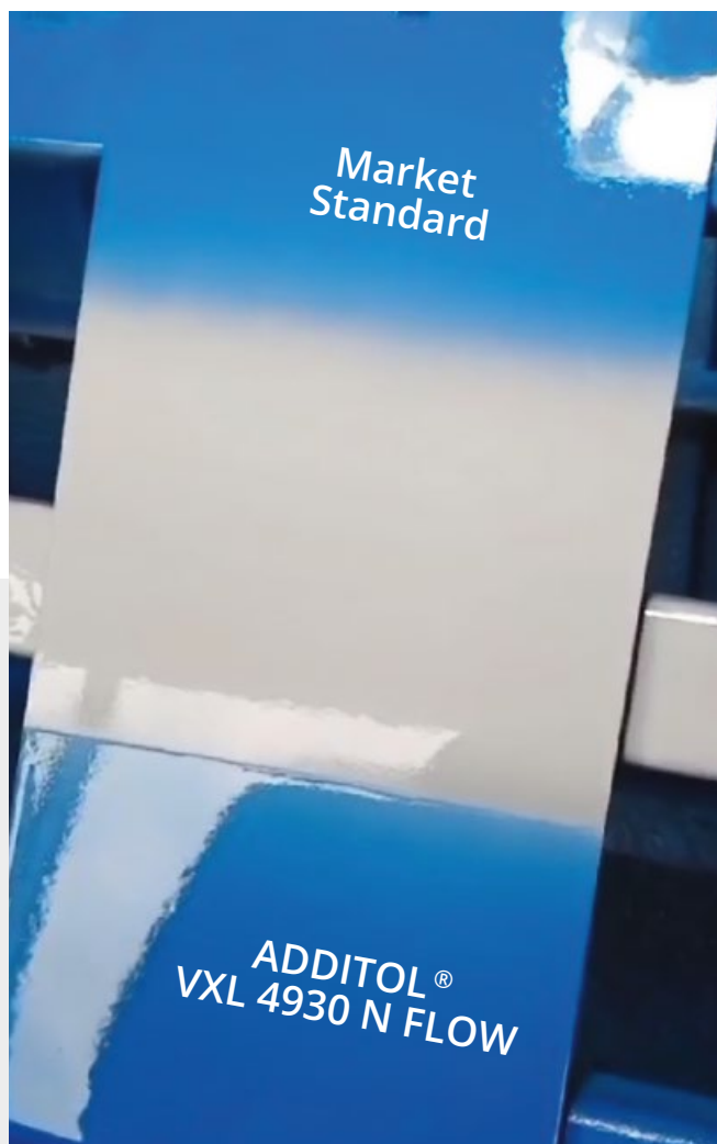
Spray dust absorption with/ without ADDITOL® VXL 4930 N FLOW
