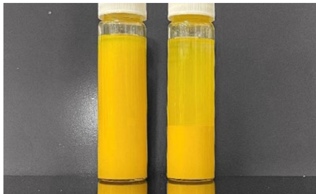
Phase separation with/without ADDITOL® XL 270 DISP
