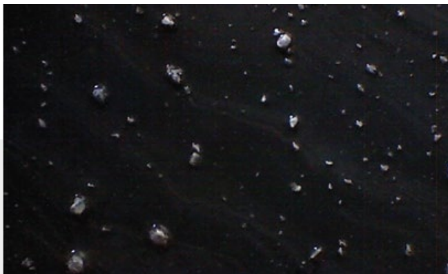
Destruction of wb Epoxy formulation by ionic dispersants
